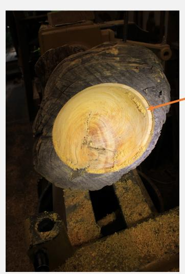
Flip it over, engage mortise on top w chuck. Pare away bottom until base is solid and flat. Make deep mortise in bottom in hard, dry wood. Engage tailstock as long as possible.
