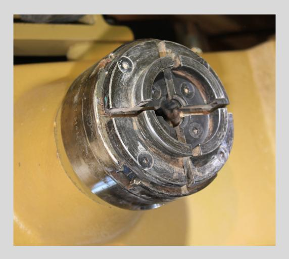
The venerable self-centering, screw operated, mechanical chuck
