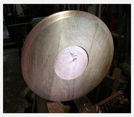
1/8" deep mortise holds well if large diameter, tight circular fit, accurate dovetail, and sound wood. Secure w tailstock
