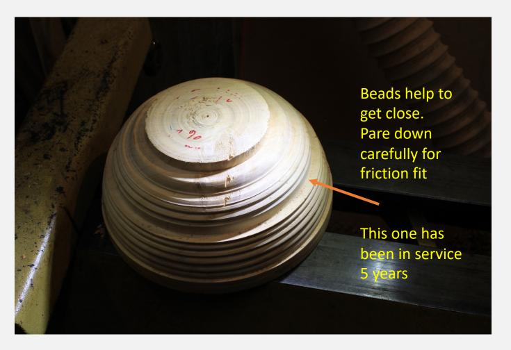
This jam chuck has a tenon on the small end, mortise on the large, for versatility<sub>105</sub>
