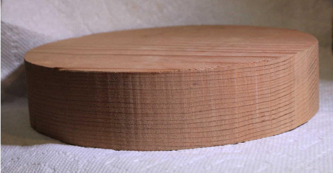
Tangential cut, 8" diameter, tightly spaced growth rings, from a very large tree. Might get away with this one as a block for a big platter, but better destiny a bowl!
