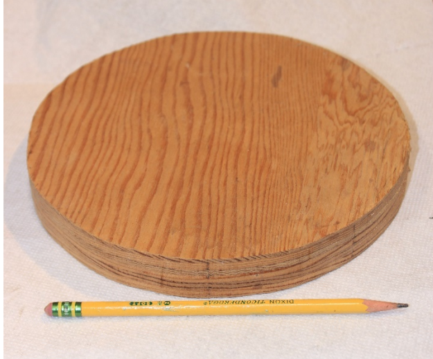
1.25" Subfloor ply, stored well, sound
