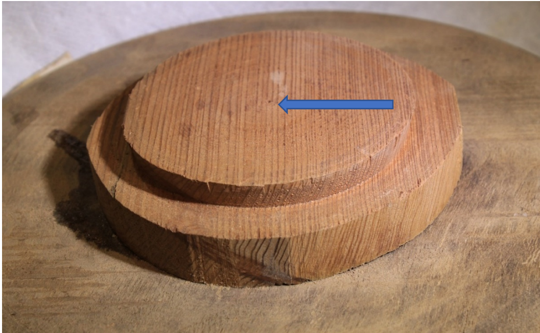
Quartersawn block with formed tenon and center awl punch. Original growth, tight grain redwood without defects...probably OK!
