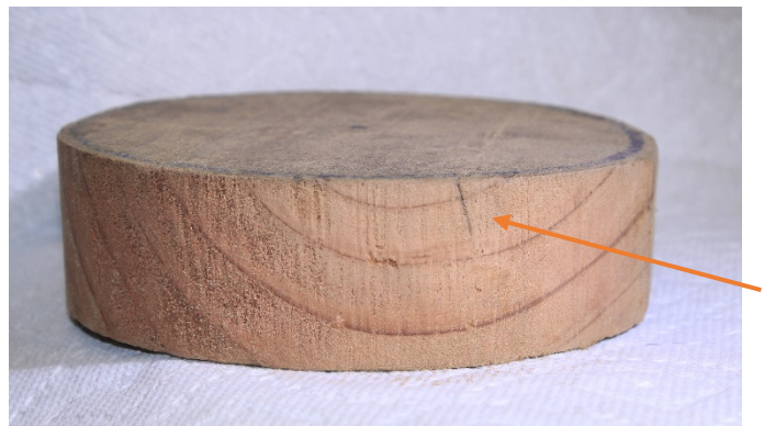
Tangential cut redwood 2nd growth/unreliable 1/2" growth rings of soft/punky wood + a crack Almost certain to fail under stress
