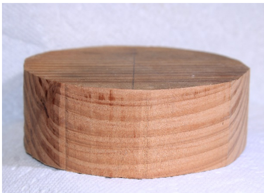
Tangential cut (D = 4") Possibly durable enough for a lightweight little bowl
