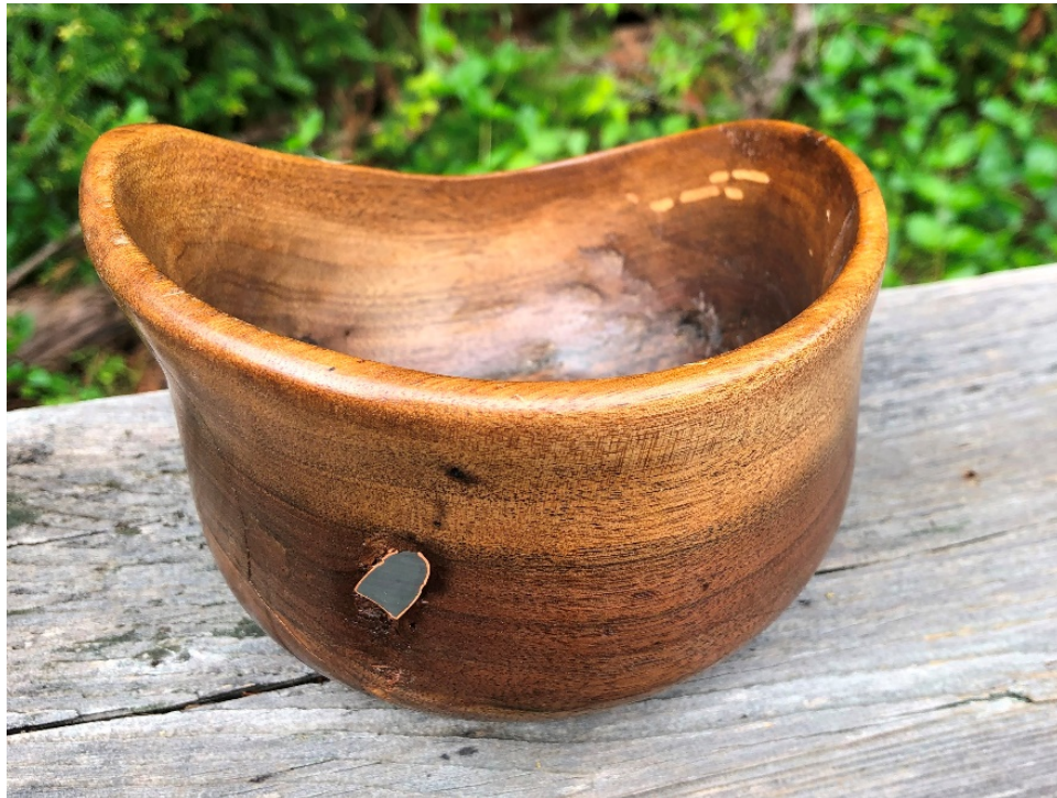
Large bore rifle bullet in Sue's Ballistic Bowl Copper jackets and lead turn nicely with a sharp HSS gouge.
