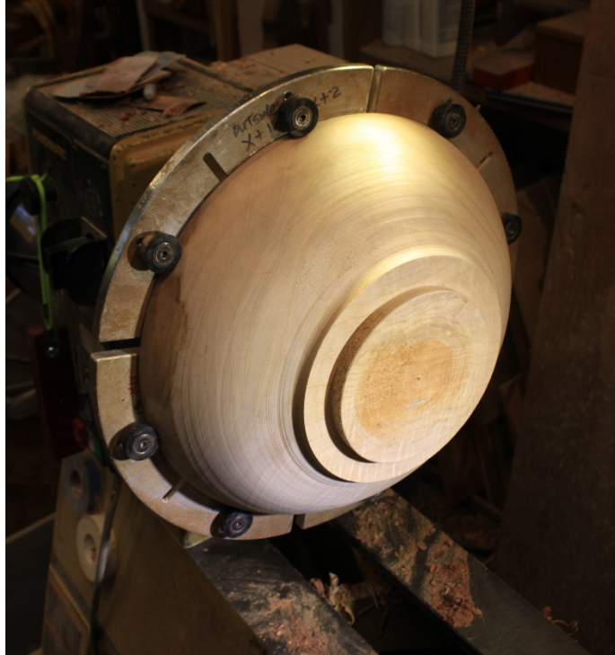
Large blank on "jumbo jaws" ready to finish bottom Tailstock would be smart! Questionable security otherwise.
