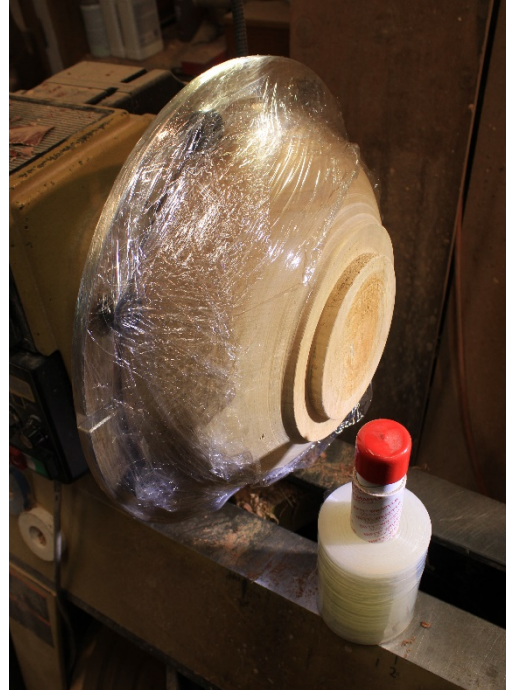
5-6 wraps → good security "Criss-cross" layers to engage both blank and back support or jam chuck
