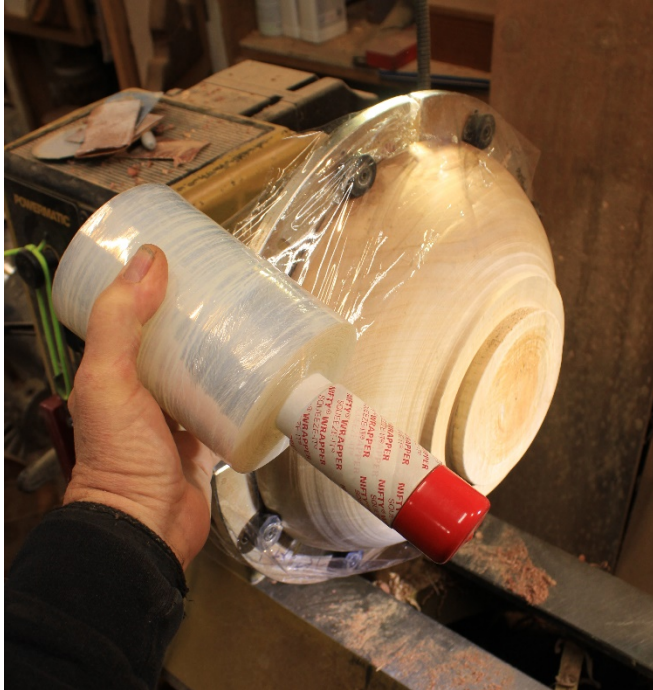
Start the wrap. (Hard to do holding a camera!) Stretch it a bit to make it conform
