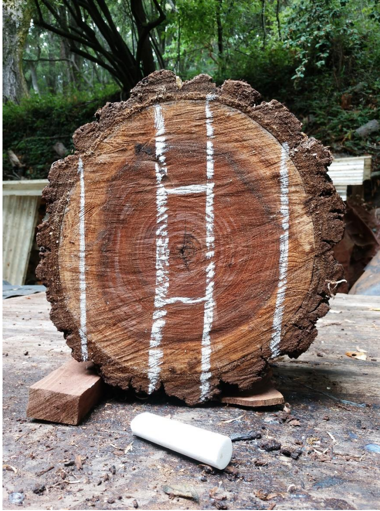
This is where we cut...over and over...deleted center pith goes for BTU's
