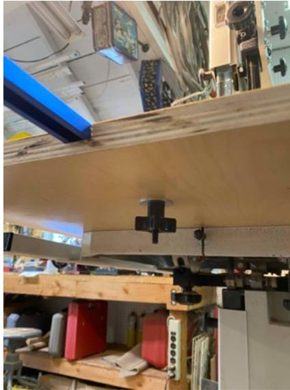
To keep the jig stable, I added a small clamp in the corner. Using an elevator bolt here again. I place some paper gasket as to not damage the saw channel. Clamp was made from steel stock.
