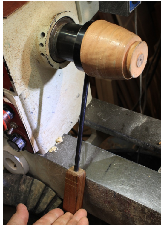
Screw chuck fixed against the ways
