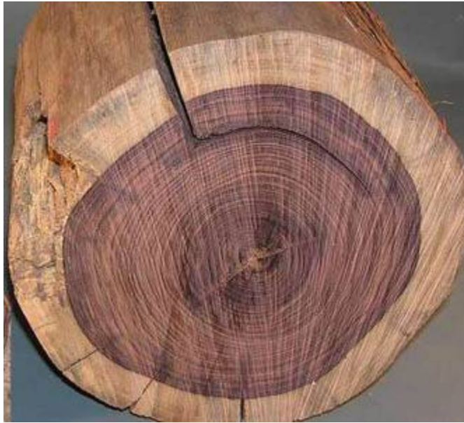
Ring shake. Ballistic liability. (Internet image) You've seen this, I know.
