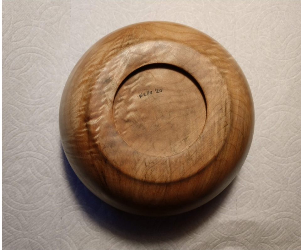
Bottom view: 2.5 inch diameter mortise with 3/4 inch rim in an 8" diameter, 5" deep maple bowl . WS
