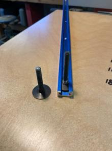
Tightening screw from the underside. Note drilled hole in center of channel for this bolt post.
