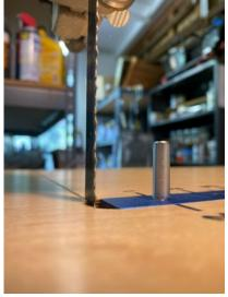
The test piece: After drilling a center hole, you place it on the pin, fire up the saw and rotate.
