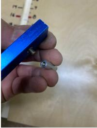
I then used an elevator bolt for riding in the T-bar and securing for a set radius of a bowl blank. As you can see, I shaved off the sides to fit the T. This also keeps it from rotating as you tighten from the underside.
