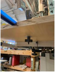
To keep the jig stable, I added a small clamp in the corner. Using an elevator bolt here again. I place some paper gasket as to not damage the saw channel. Clamp was made from steel stock.
