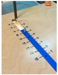
I also made sure the center of the post is in line with the cutting, front edge, of the bandsaw blade. Not sure if this is right. This seems to work and not bind as I cut.
