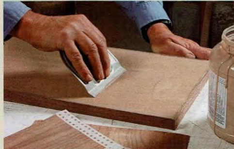
Trowel is better than a roller. A spreader with \frac{1}{2} -in. V-notches will deposit the perfect amount of PVA glue for veneering and laminations.
