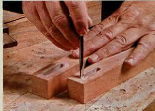
Reach into mortises. Squeeze glue into the mortise, and then spread it with the brush. Glue is not necessary on tight-fitting tenons.
