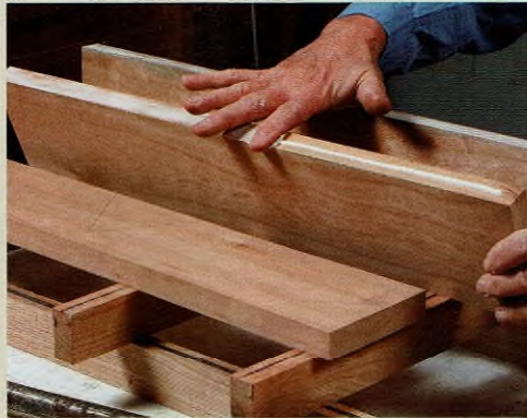
The simplest spreader. Fortune uses his finger to spread the glue on edge joints, bending it a bit to get more glue in the middle than along the edges.
