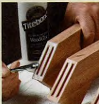
Miter master. On end grain, this glue stays on the surface longer, giving you more time to complete the glue-up.
