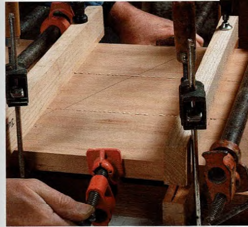
Don't apply too much. On clamped joints like panels (left) and miters (above), you should see a small continuous line of squeeze-out. Big beads or drips will be harder to deal with afterward.
