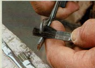
Doctor it first. Trim the bristles on cheap flux brushes to make them stiffer, and hammer the ferrule to keep the bristles from falling out.
