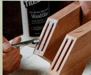
Biscuits and miters, too. The brush reaches into biscuit slots and spreads glue on small surfaces like these miter joints.
