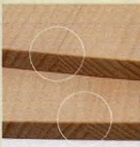
Perfect for pine. The glue line is dark (top) using Titebond III, but invisible (bottom) using Titebond Extend.
