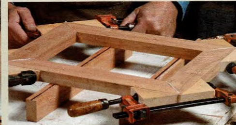
Don't apply too much. On clamped joints like panels (left) and miters (above), you should see a small continuous line of squeeze-out. Big beads or drips will be harder to deal with afterward.
