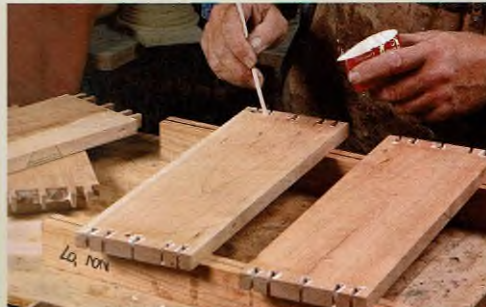
Dovetail trick. Thin sticks reach between tails to apply a thin, even coat. You don't need glue on the pins, but a little on the shoulders doesn't hurt.
