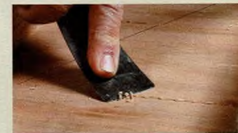
Don't apply too much. On clamped joints like panels (left) and miters (above), you should see a small continuous line of squeeze-out. Big beads or drips will be harder to deal with afterward.
