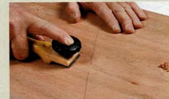
After about an hour, remove the clamps and get the rest of the gummy squeeze-out with a cheap, steel-bladed paint scraper (bottom). Grind a fresh edge on each tool for best results, and ease the corners so they don't dig in.
