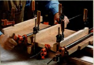
Got 15 minutes? Standard PVA glue has a relatively short working time, but it's more than enough for many glue-ups. Always do a dry run to get everything set before spreading glue.
