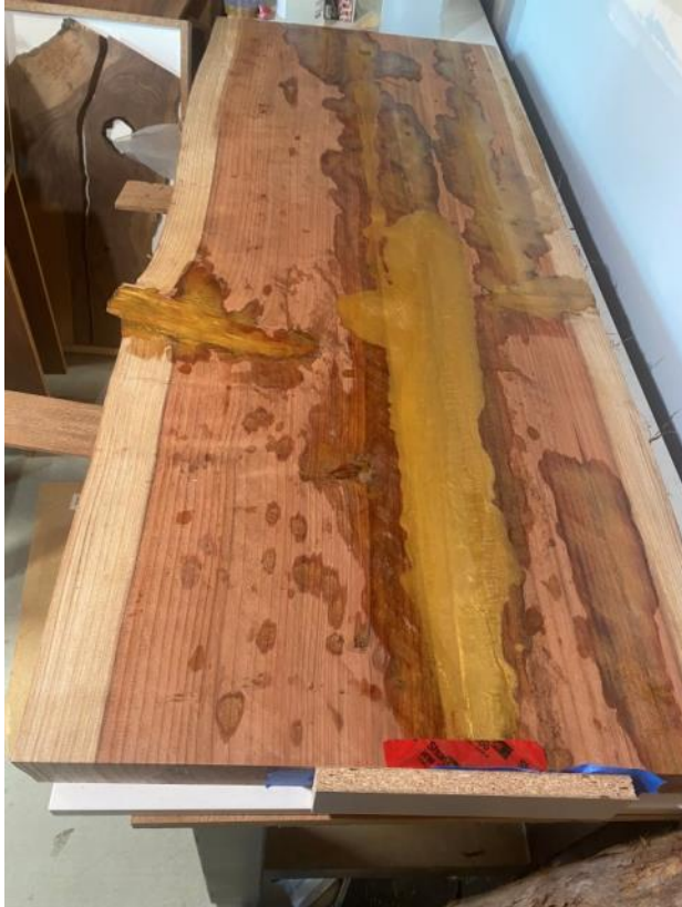
Redwood countertop getting epoxy stabilization of crack in center and vulnerable knot.
