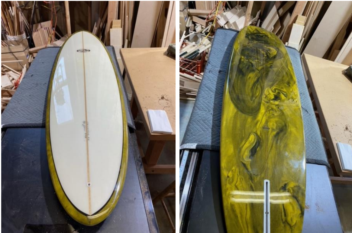
Resin finished surfboard top and bottom. "Acid Swirl" pattern colors embedded in lamination process. Mattie Guthrie
