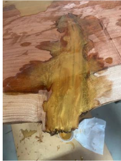
Redwood countertop getting epoxy stabilization of crack in center and vulnerable knot.
