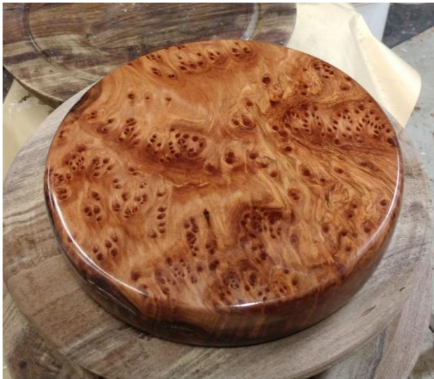
Redwood burl initially with many voids and perilously unstable "wafer" cracks, solidified with slow set clear System Three epoxy (2 days immersion), turned, and finished. WS
