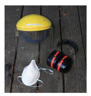
**Good face shield** is essential. Polycarbonate glasses with side shields have advocates as sole protection, but as soon as you rough out a big blank and hear the hail of shavings rattling off your shield like gravel on your windshield behind an uncovered truck on Hwy 17, you'll want full face protection.
