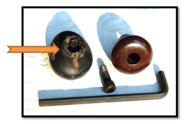
Using the lathe to turn a new handle out of walnut left over from a table leg project, and the tailstock chuck to counter bore the wooden one with a 3/8" shaft hole and a 5/8" access, I came up with a functional facsimile.
